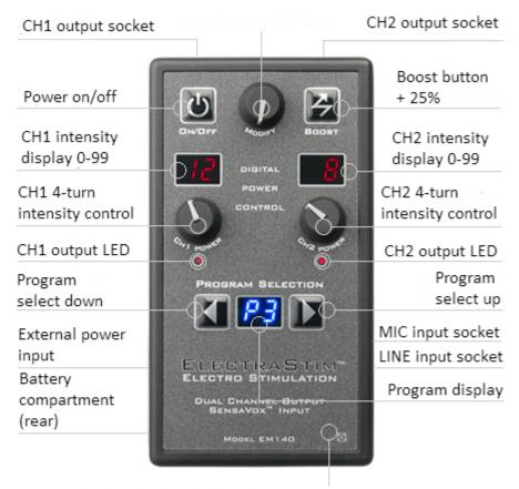
Durable reverse printed polycarbonate overlay with easily locatable embossed control buttons
