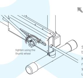
Set the desired thrust rod length and tighten using the thumb wheel.
